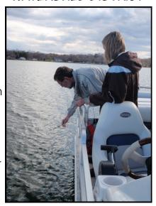
A secchi disk is a weighted circular metal disk, 8 inches in diameter, attached to a rope marked for measurement. The disk is black and white or all white in color. To collect a secchi disk measurement, the disk is lowered into the water column until it disappears. The secchi depth is measured by recording the depth at which the disk reappears. Deeper secchi disk readings (larger numbers) indicate clearer water.
